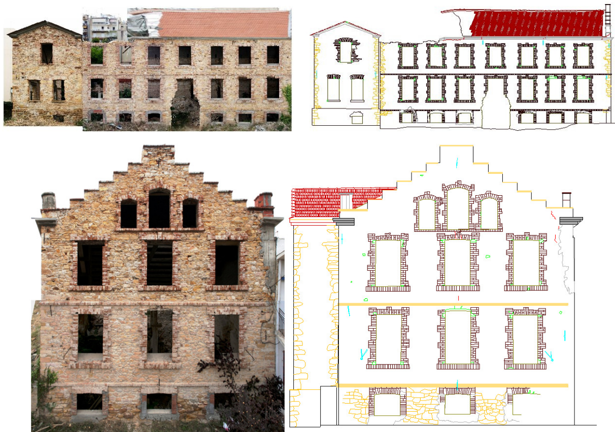
Figure 5: Rectified mosaic of images (left) and corresponding digitized façade (right) of the western and the southern façades of the partially-collapsed tobacco warehouse in Alexandroupolis
