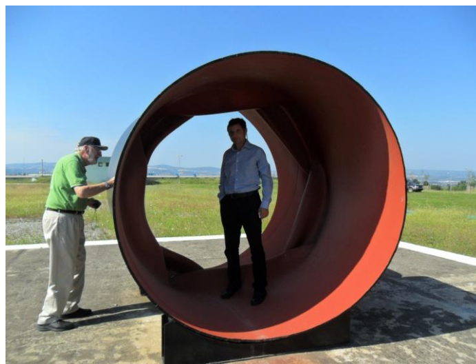
Figure 1. A close-up view to the wrinkled pipe in Kullar, Izmit during the 1999 Kocaeli Earthquake
