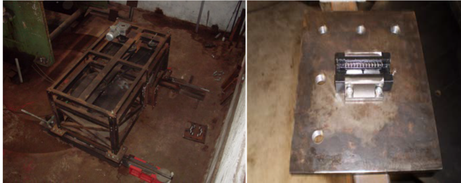
Figure 6: Vibrodyne on the guides.
