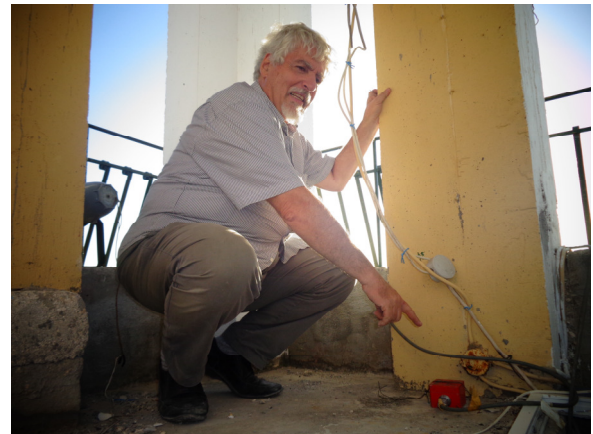
Figure 17-18. Accelerometer fixed at “High Measuring Point (up)”.
