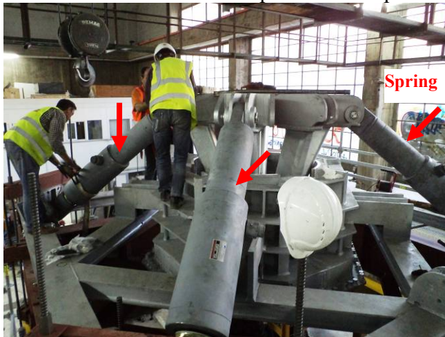
Figure 15. Four springs connecting the four top corners of the sliding core to the four corners of the 3-D square steel rigid frame of a suspension unit.
