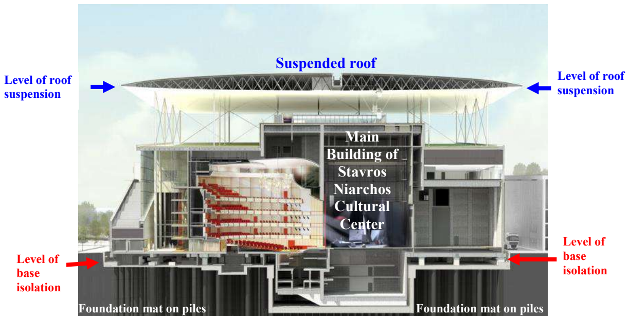
Figure 1. The Stavros Niarchos Cultural Center. The main building is supported on a base isolation system formed by inverted pendulum bearings. The suspended roof supported on slender hollow steel columns.
