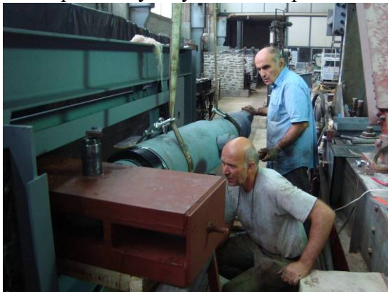
Figure 19a. Spring being fitted at the loading frame
