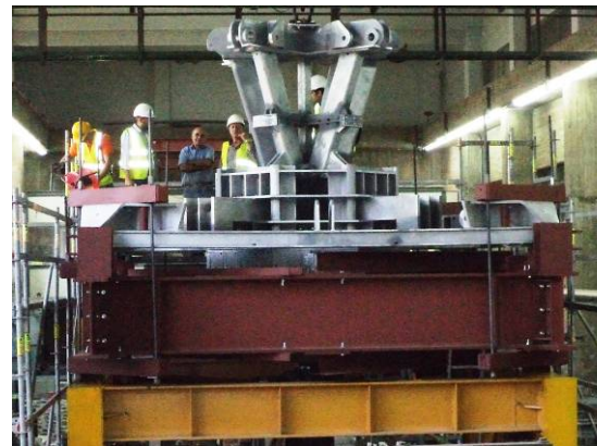
Figure 14. The rigid steel core with the sliding pads. This core slides within a polygonal rigid frame that is also visible at the center of figure 13.
