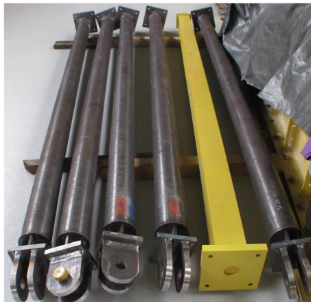
Figure 4: Conventional brace (yellow color) and buckling restrained braces
