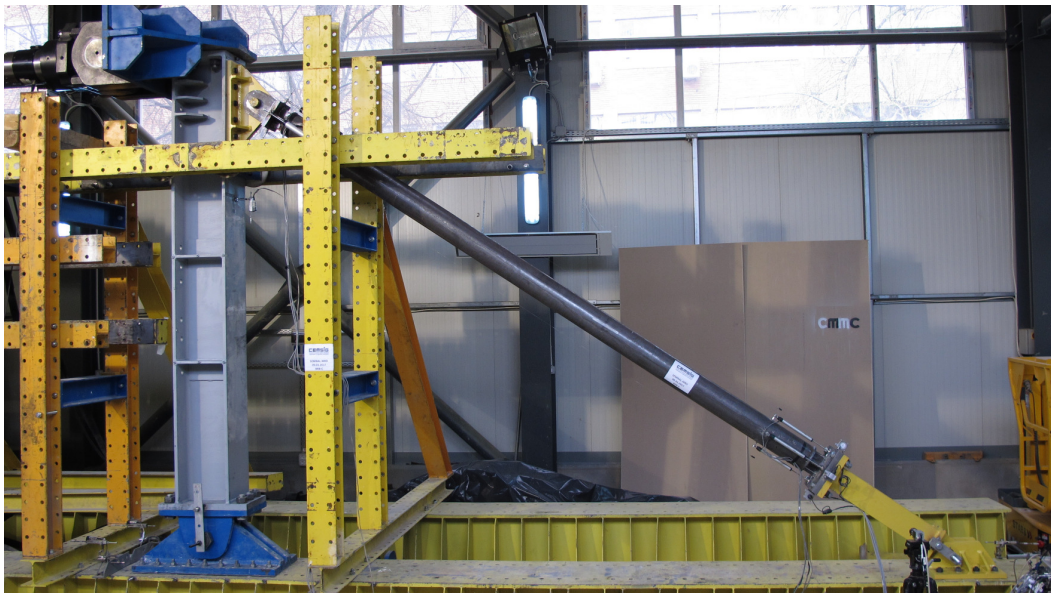
Figure 8: Experimental test set-up for the investigation of the buckling restrained brace (see Figure 6a).
