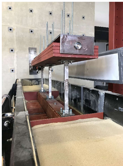
Figure 5: Experimental setup with the model on sand
