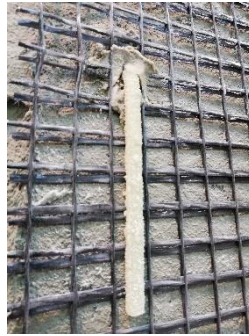
Figure 4: Specimen R2-OOP: Detail of the L-shape connector.
