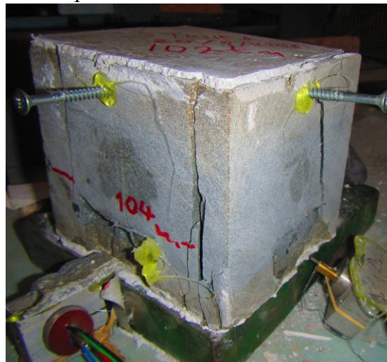
Figure 10. The failed stone specimen. Notice the dislocation of the displacement transducers and the debonding of the strain gauges at this final stage of testing.
