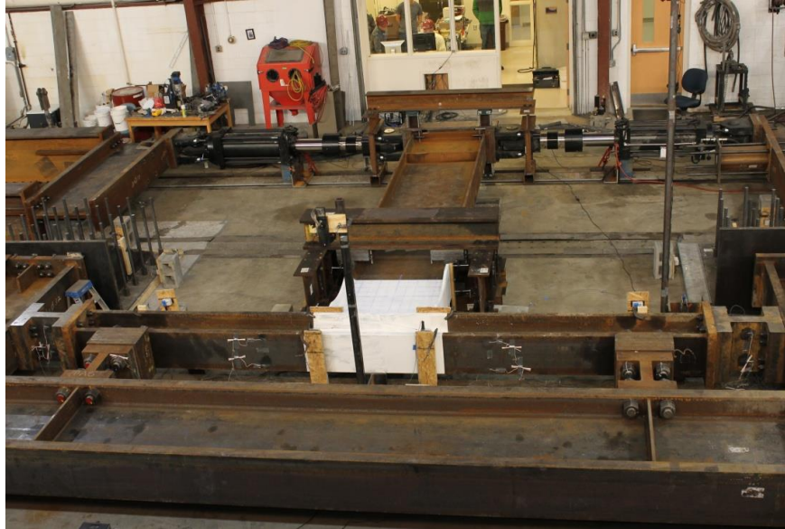
Figure 2 Specimen in testing orientation with two actuators
