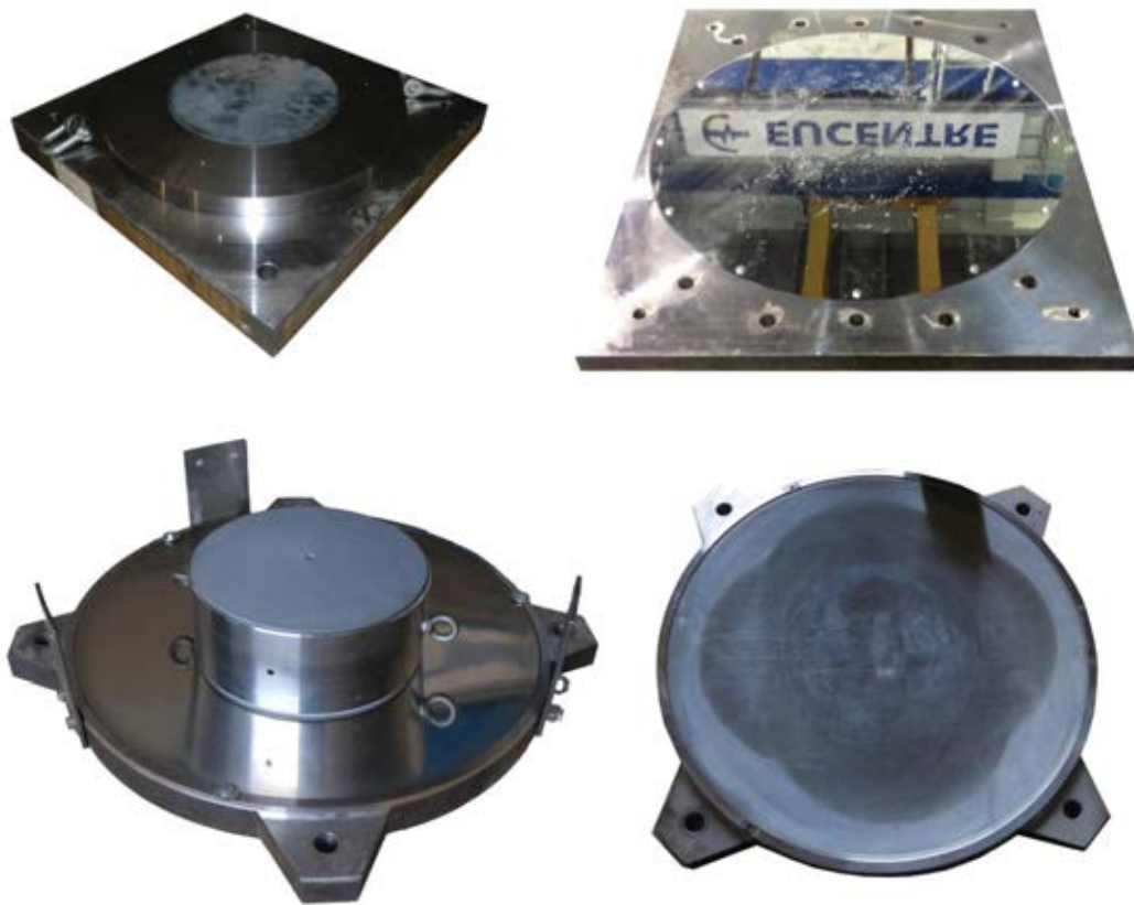
Figure 1: Full-scale Flat (top) & Concave (bottom) Surface Slider devices (FS & DCSS)
