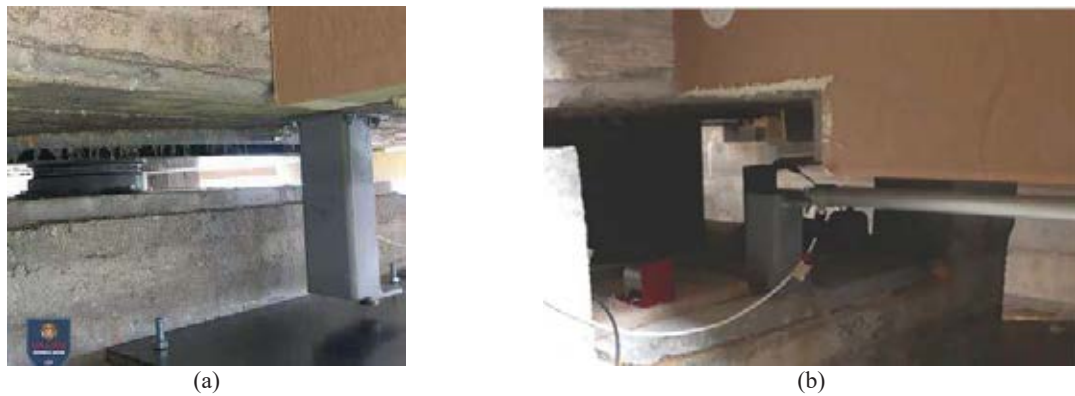
Figure 7: Sensors for recording vertical (a) and horizontal (b) displacements.
