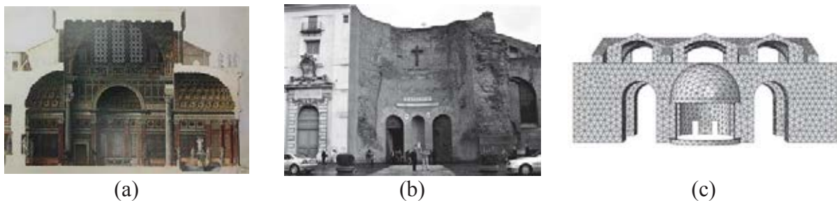
Figure 6: Baths of Diocletian: (a) transversal cross-section of the Calidarium (E. Paulin, 1880), (b) current state, and (c) FE model
