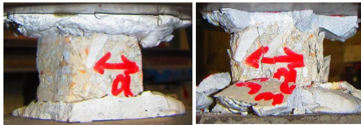
Fig. 15. Compressive test of a concrete sample taken from the bell tower columns ( f_c=21.2\text{MPa} )
