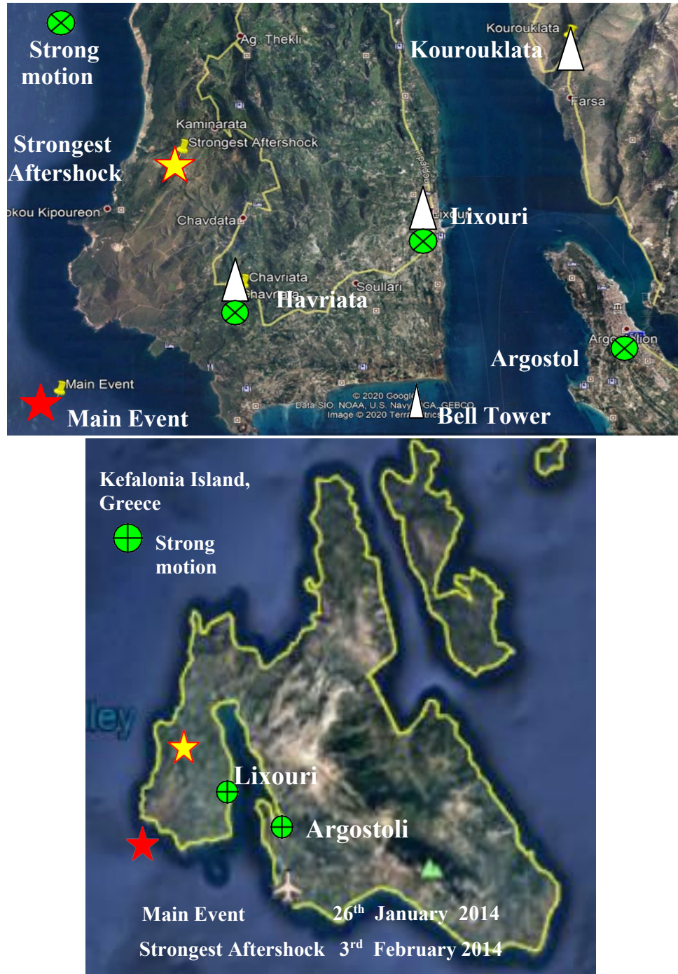
Figure 10. The location of the epicenters, the bell towers and the instruments that recorded the earthquake strong ground motion
