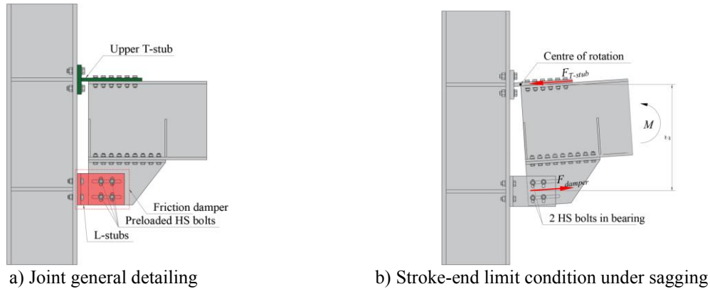
Figure 2: Particularities of FREEDAM joints.
