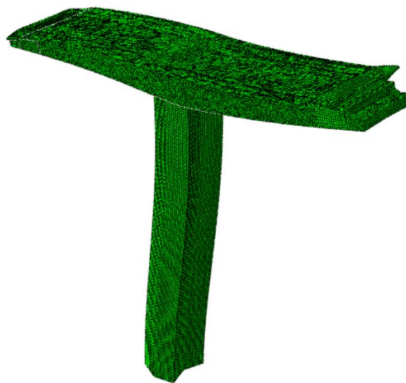
Figure 23: 1th Eigenmode ( f=1.435 Hz) translational along the vertical axis
