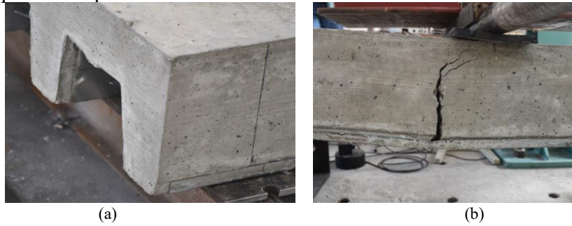
Figure 4: (a) Debonding at F_{max} and (b) flexural cracking of the concrete at the end of the tests.
