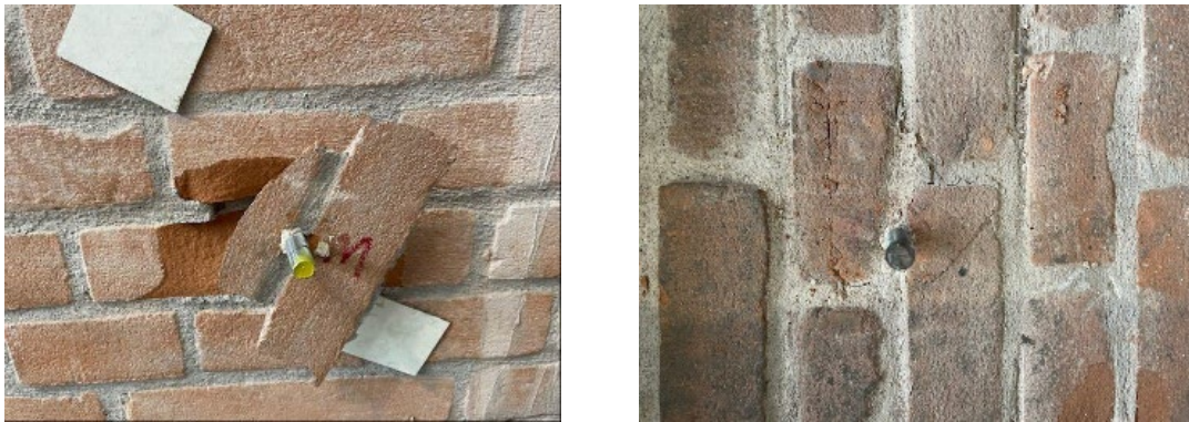
Figure 5: Failure modes for single anchor tests (left, 1A-100-0.2-W0-3; right, 1A-100-0.2-W3-7).
