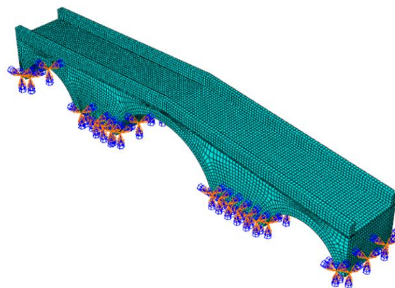
Figure 5: Numerical model and boundary condition.
