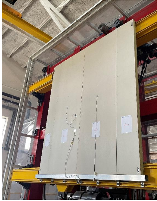
Figure 2: View of the façade system with sandwich panels specimen.
