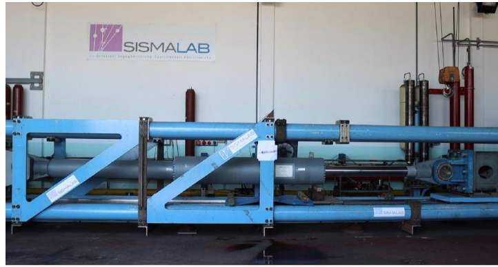
Figure 5: Picture of the damper type MHD4400kN
