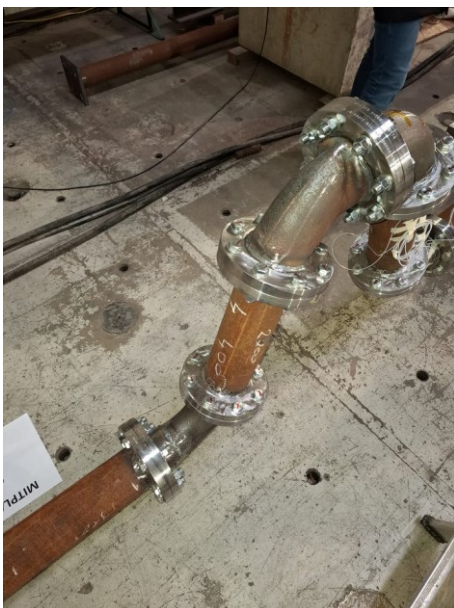
Figure 18 Final state of the pipe with the flanged Omega joint.
