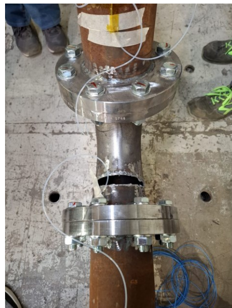
Figure 18 Final state of the pipe with the flanged Omega joint.
