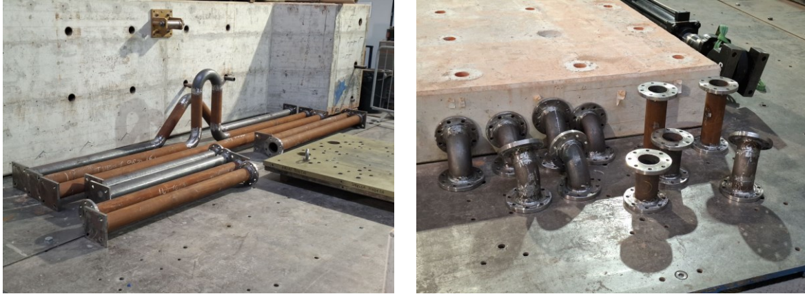
Figure 1 Example of the pipeline configuration specimens.
