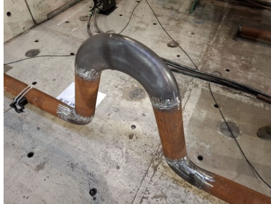
Figure 16 Final state of the pipe with the welded Omega joint.
