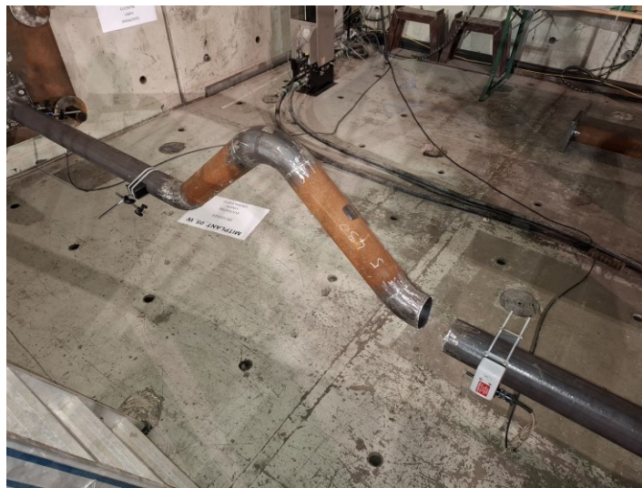
Figure 17 Final state of the pipe with the welded V joint.
