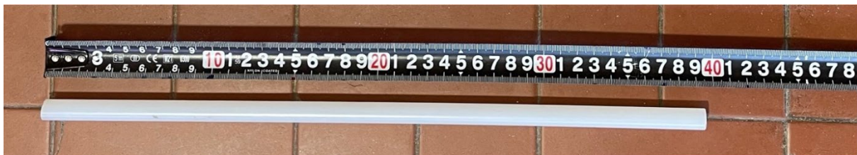
Figure 2: Smooth nylon bar before the laboratory test.
