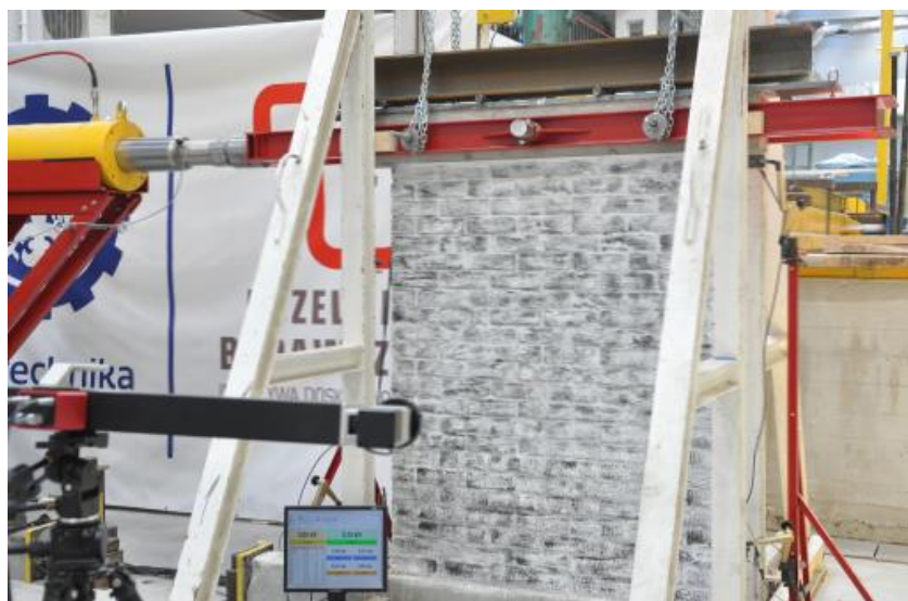
Figure 2: Camera position for the DIC system.
