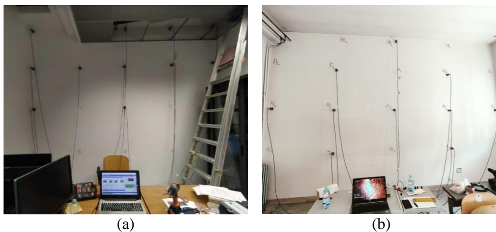
Figure 3: (a) 15 cm-thick and (b) 37 cm-thick partition walls tested.
