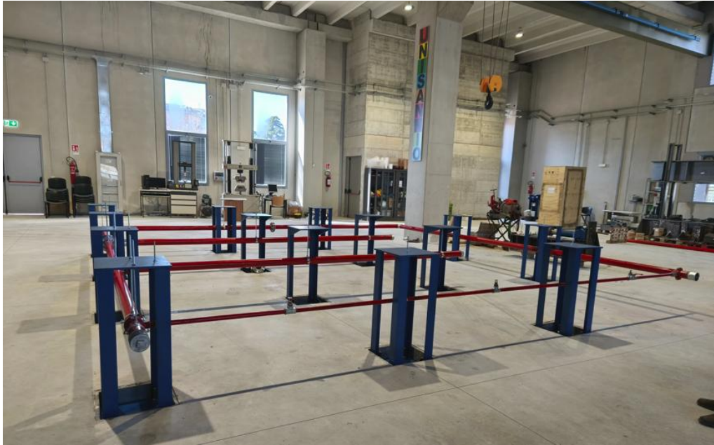
Figure 4: Fire protection piping system under test.
