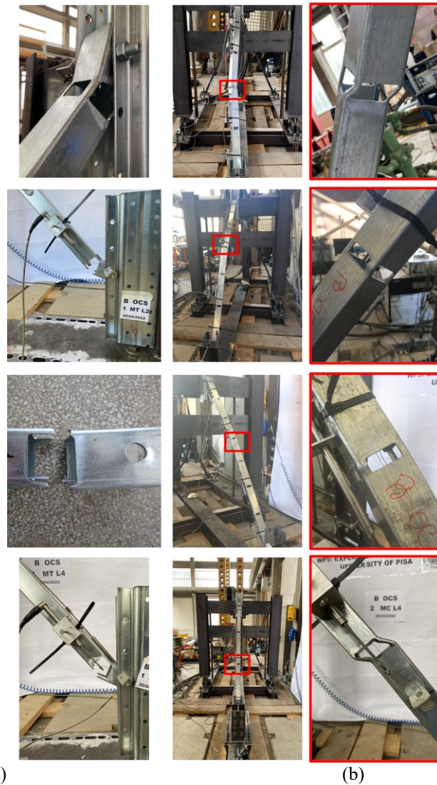
Figure 4: Failure of the elements under monotonic (a) tensile and (b) compression load.
