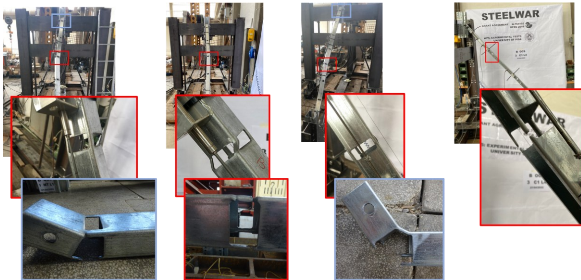
Figure 6: Failure of the elements under cyclic load.
