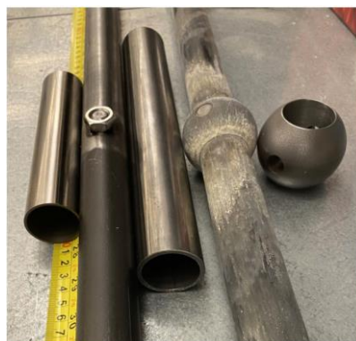
Figure 2: Piston rods used in the pressurized sand damper where the mounted sphere has been replaced with a 1.27 cm diameter bolt. (Adapted from [11].)
