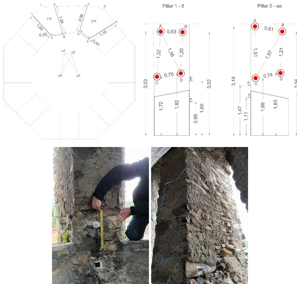
Figure 8: Instruments location over the pillars.
