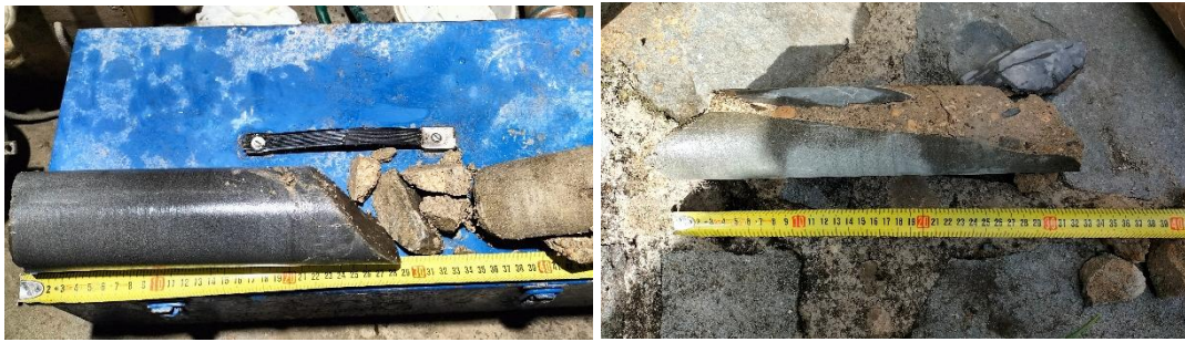
Figure 2: Drilled core samples.
