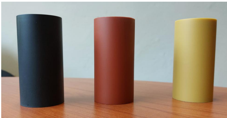
Figure 2: Polyurethane gel samples tested in this work: height 100 mm, diameter 50 mm.
