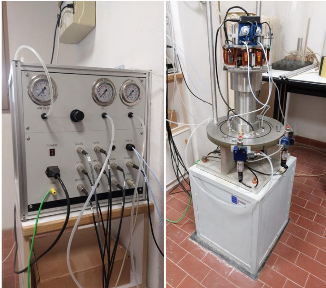
Figure 3: Resonant Column and Cyclic Torsional Shear Tests Apparatus.
