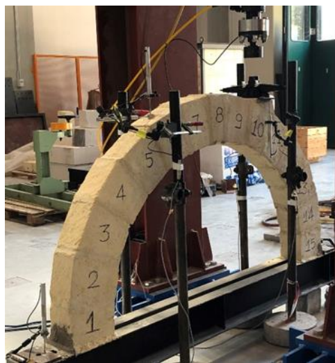
Figure 1: Geometric configuration of the arch and LVDT (P1 – P6) position.
