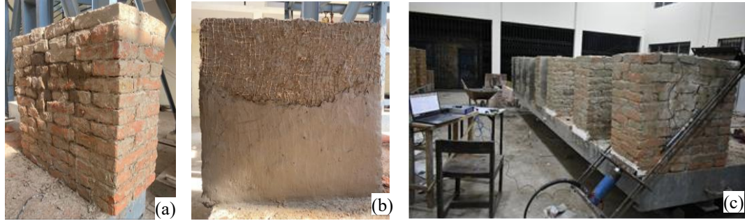
Figure 5. Prepared wall panels (a) without render (b) render with jute fibre and fibre mesh (c) test setup.
