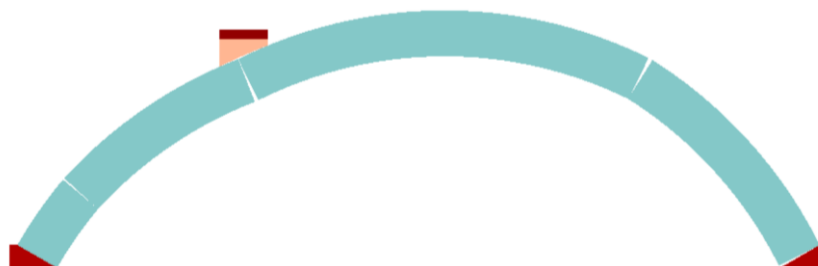
Figure 11: Numerical failure mechanism observed in the arch with weak masonry strengthened using FRCM ( Planitop Intonaco Armato ).
