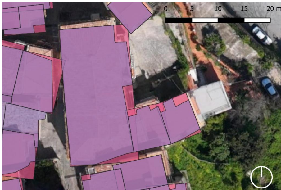
Figure 2: Zoom on a portion of a historic urban center: view of the polygons representing buildings from cadastral maps (dark purple) and corresponding minimum oriented bounding boxes (light purple).
