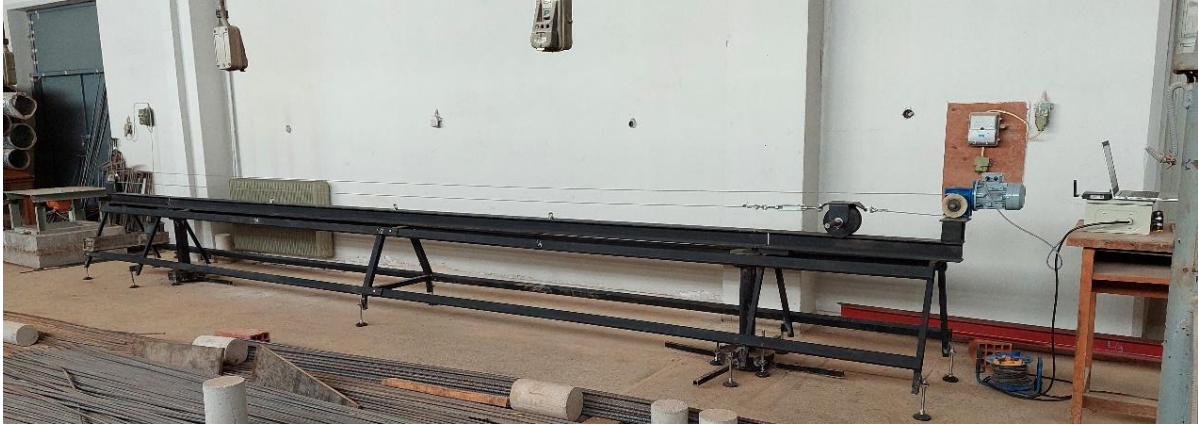
Figure 1: Experimental setup for moving mass tests.
