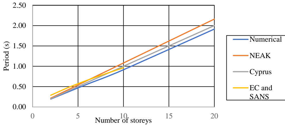
Figure 10: Relationship between period along the y-direction and number of storeys for the initial models with shear walls.
