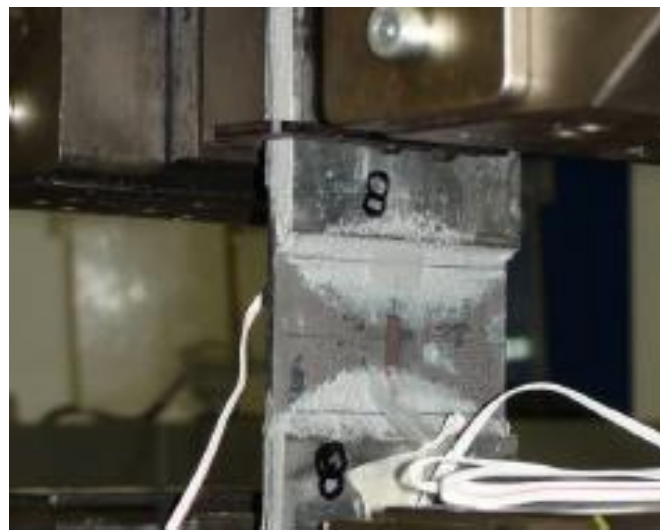
Figure 7: Test set-up for the tension test
