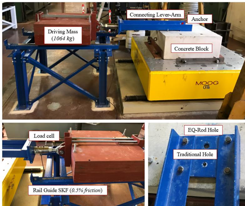
Figure 3: Details of shake-table test setup.
