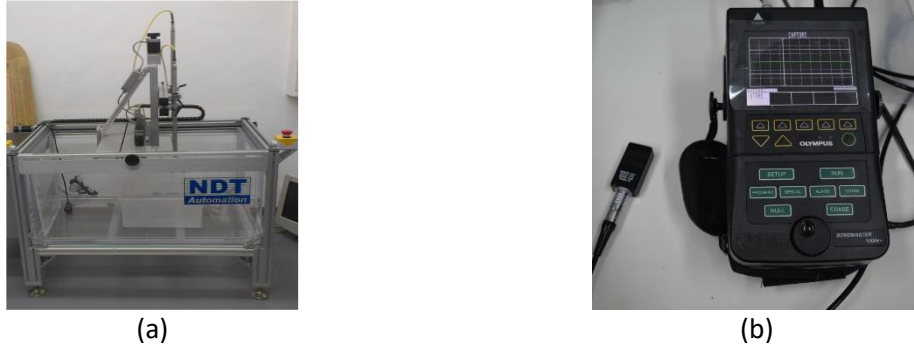
Figure 11: Non destructive testing apparatus. (a) Ultracac II by Mistras Group. (b) Olympus Bondmaster.
