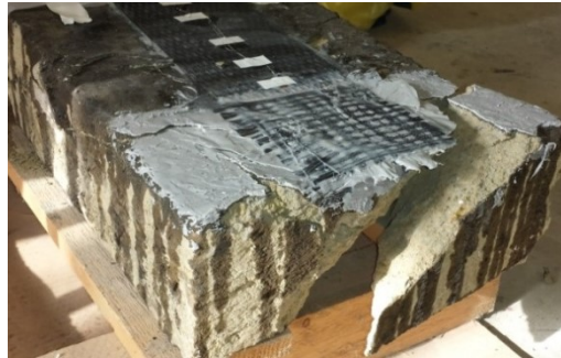
Figure 5: Failure surface at the end of anchored specimens made of tuff stone (Ceroni, 2017, [7]).
