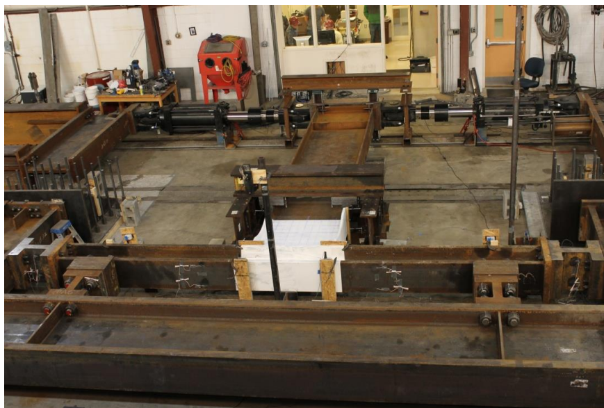
Figure 2 Specimen in testing orientation with two actuators
