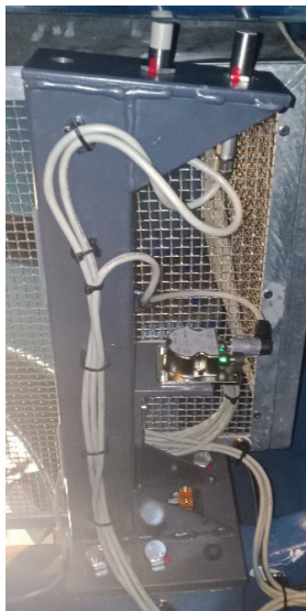
Figure 8: Combination sensor holder
