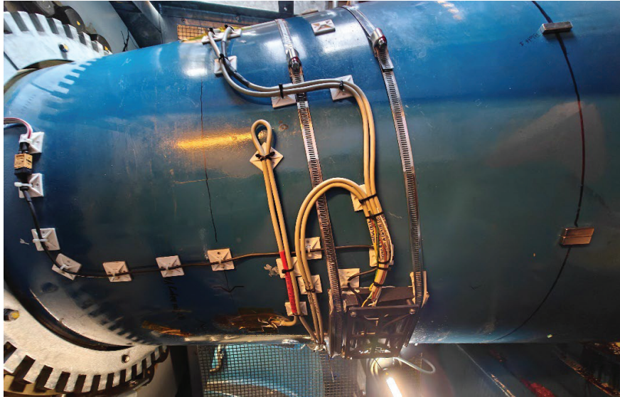
Figure 7: Instrumented rotor shaft
