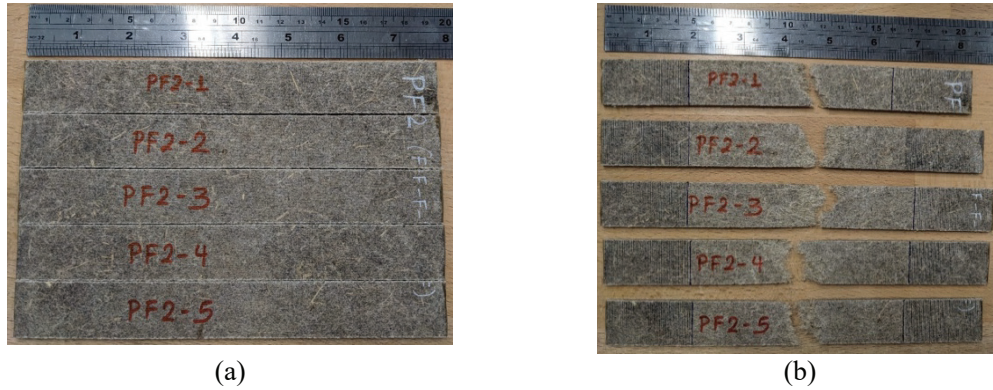
Figure 2 Five tensile samples cut out of panel PF90 after the water immersion for 90 hours (a) samples before tensile testing; (b) samples after tensile testing.
