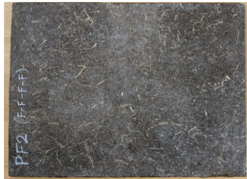
Figure 1 Flax reinforced panel straight after fabrication, in dry condition.
